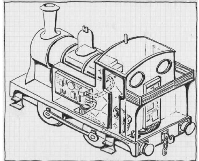
[7] Phantom view of Connoisseur O Gauge tank engine with relative positions of Decoder, Battery, BPS and Motor.
