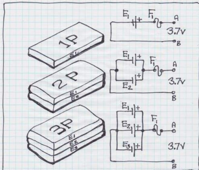
[40] Schematic showing battery with identical cells in parallel. Adding more cells does not increase the terminal voltage between A and B.
