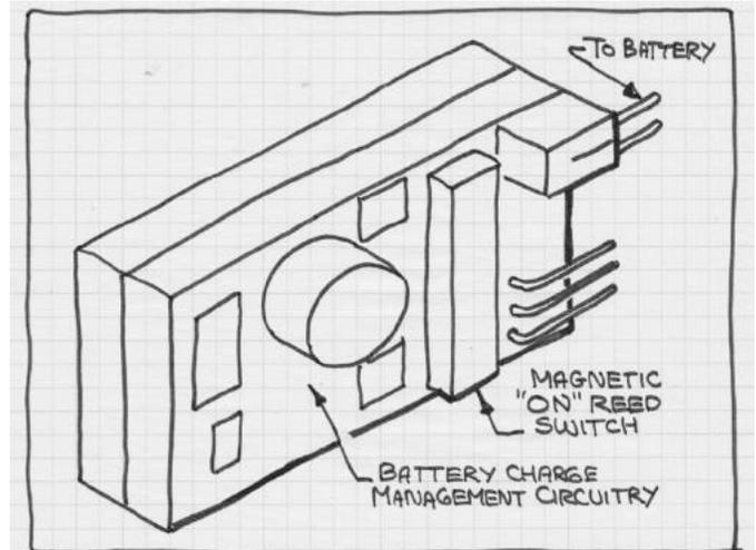
[19] Magnetic reed "ON" switch location on BPS. This has to be close to the loco's surface.
