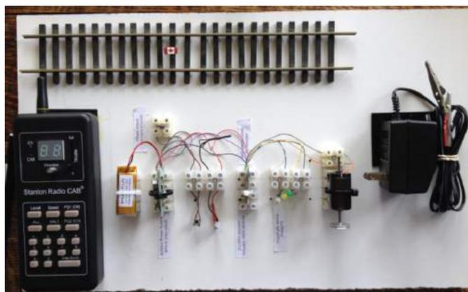
[16] Test set-up to evaluate the parts working together before wiring into the loco.
