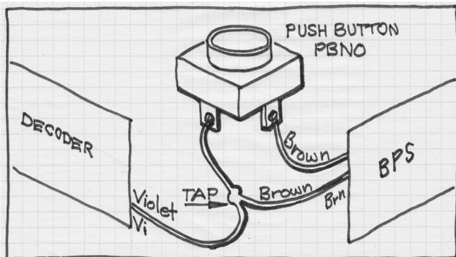
[13] Illustration for PBNO wiring to push Battery OFF but still enabling S-CAB transmitter OFF.
