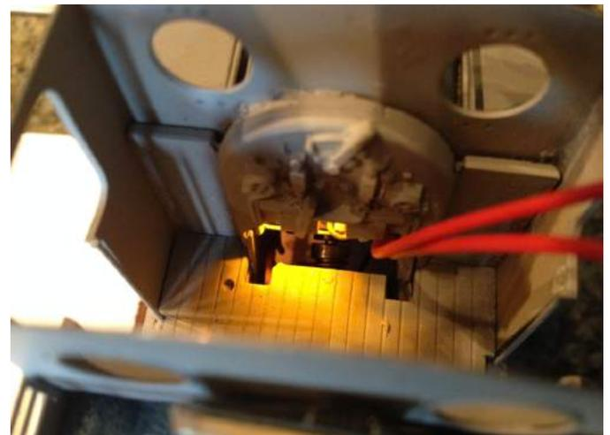
[46] Boiler fire as represented by two flickering candle LEDs and intended as a power-ON indicator. The two red wires are connected to the battery for performance tests.
