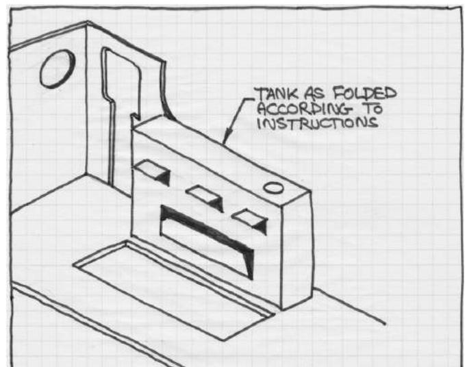
[20] Loco side tank before mutilation showing the rectangular hole on the inside of the water tank, which had to be made larger.
