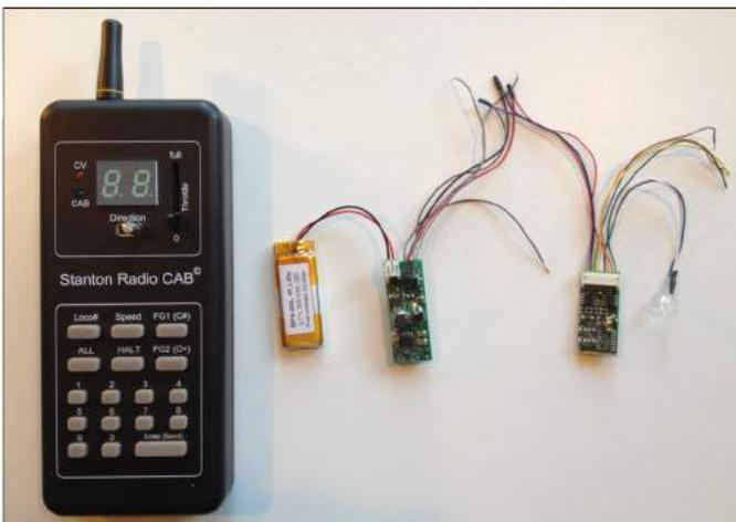
[1] S-CAB controller and parts for locomotive: LiPo Battery, Battery Power Supply controller and Radio Receiver Decoder.
