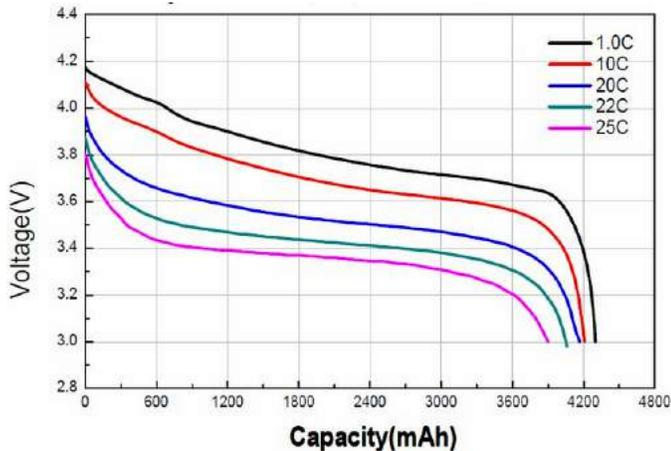
[37] *LiPo batteries change voltage as they discharge over time. The voltage also drops as the current increases.*
