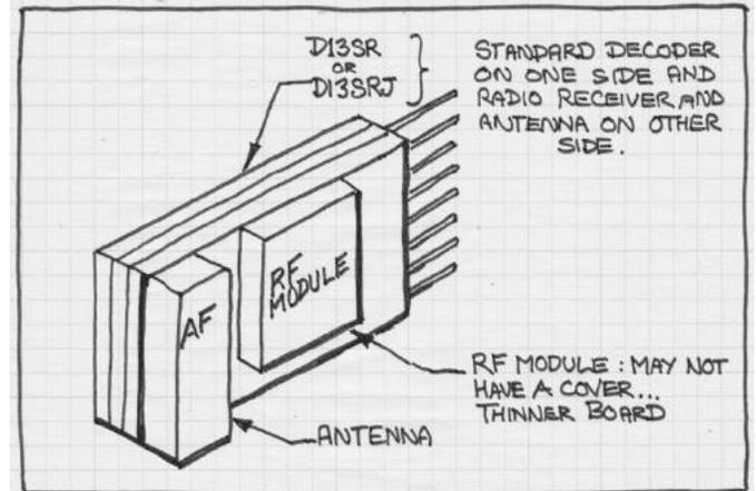
[28] Antenna (AF) location on the NCE radio Decoder. This works best with a clear line of sight but works reasonably well with obstruction.
