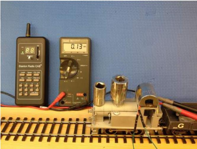
[50] Set up to test current draw at differing wagon loads and grades.
