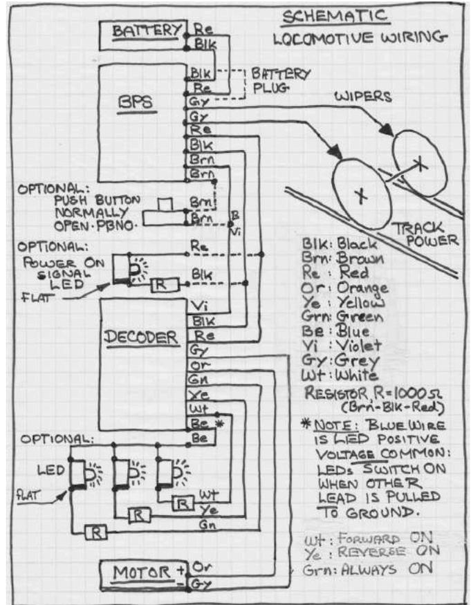
[15] Complete tank loco S-CAB wiring diagram.
