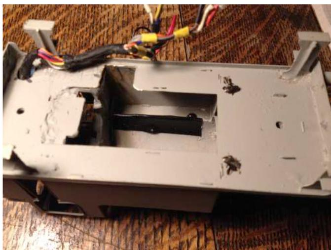
[22] Notched frame and side tank metal removed and viewed through the frame.
