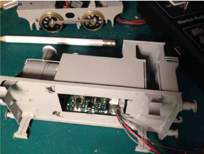
[25] BPS in side tank viewed through loco frame motor well.
