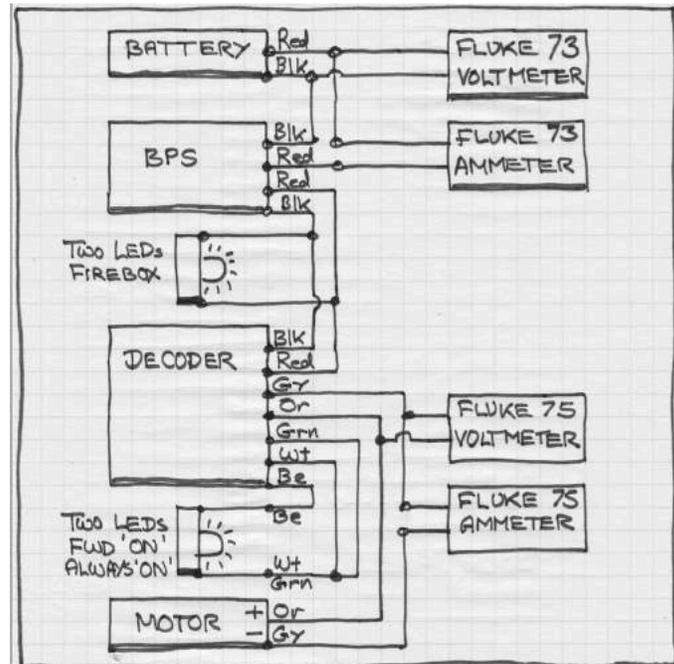
[53] Wiring diagram of Motor-Loading and current draw test set up.
