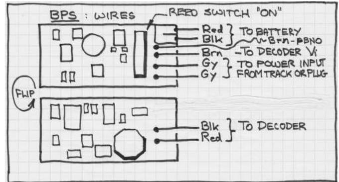
[23] Both sides of BPS with wire colours and functions.
