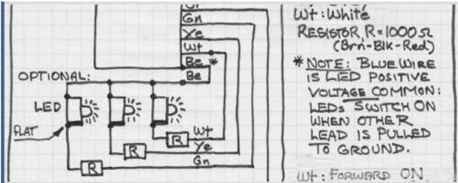
[47] Section of the complete locomotive schematic showing Decoder LEDs and wire colours.
