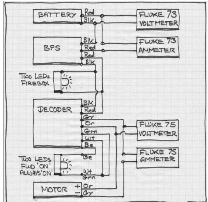
[53] Wiring diagram of Motor-Loading and current draw test set up.
