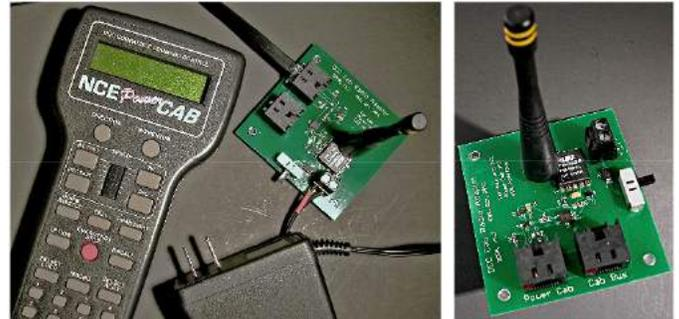
55. *The S-CAB Radio Programming Adapter (RAPA) with an NCE controller and power supply for changing manufacturer specific CV's.*
