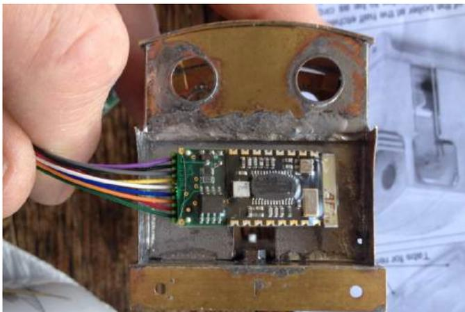
[30] Trying out the location and orientation of the radio decoder. Lots of room in the bunker but questions needed to be answered as to whether it would be shielded in this position.
