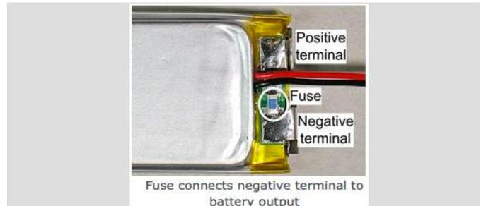
[42] Fuse location on battery ... wrapping removed. Above illustration used with permission from S-CAB.
