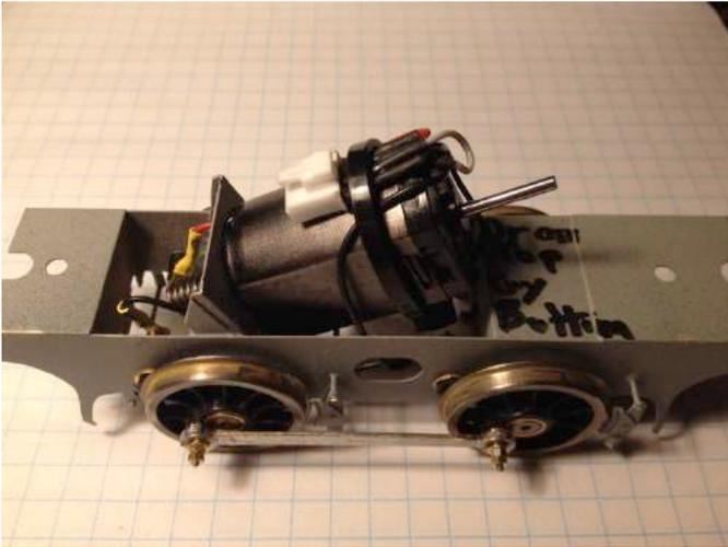
[34] Motor orientation with motor leading worm gear has wiring implications. A flywheel will be fitted after clearance is checked from the battery.
