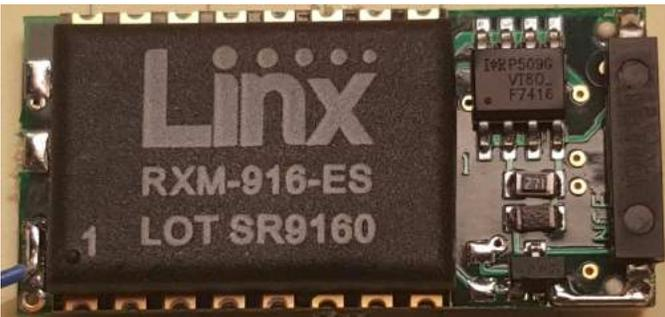
[26] Double sided radio Decoder from NCE. Radio receiver side above and decoder side below.
