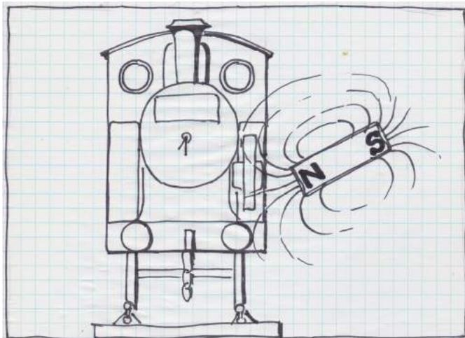
[18] Bringing a magnet close to the "ON" reed switch on the BPS turns the BPS and the decoder ON. Correspondingly, bringing a magnet close to the "OFF" reed switch turns everything OFF.
