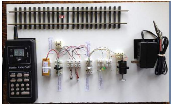
[16] Test set-up to evaluate the parts working together before wiring into the loco.
