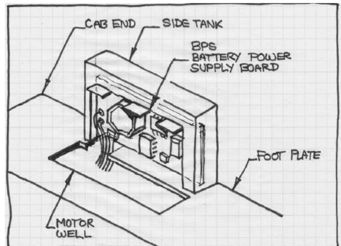
[24] BPS location in side tank with wire feed through taped notch.
