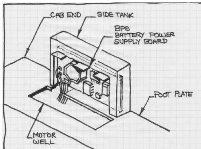
[24] BPS location in side tank with wire feed through taped notch.
