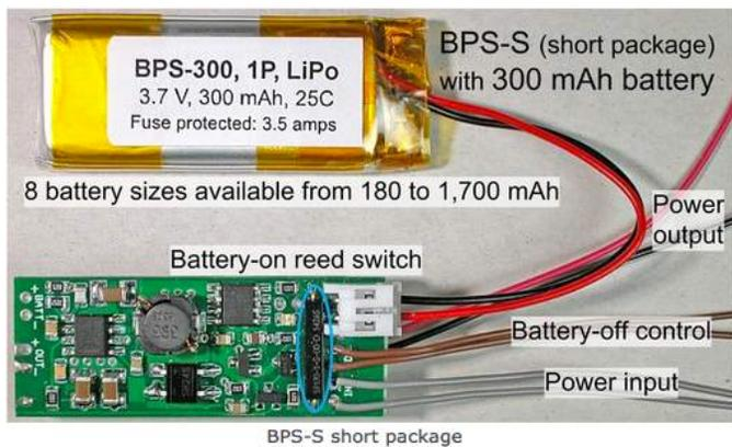
[17] BPS and Battery wiring, functions and colours. Above illustration used with permission from S-CAB.
