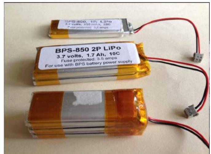
[39] *Batteries wired in parallel to increase capacity. The voltage is the same at 3.7v for all three examples.*
