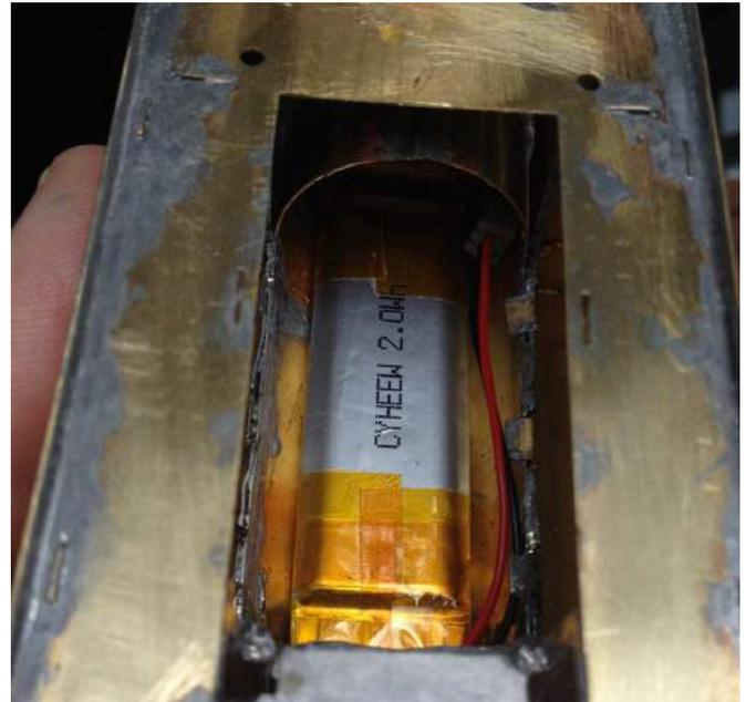
[41] Battery taped to boiler roof and viewed through motor well.
