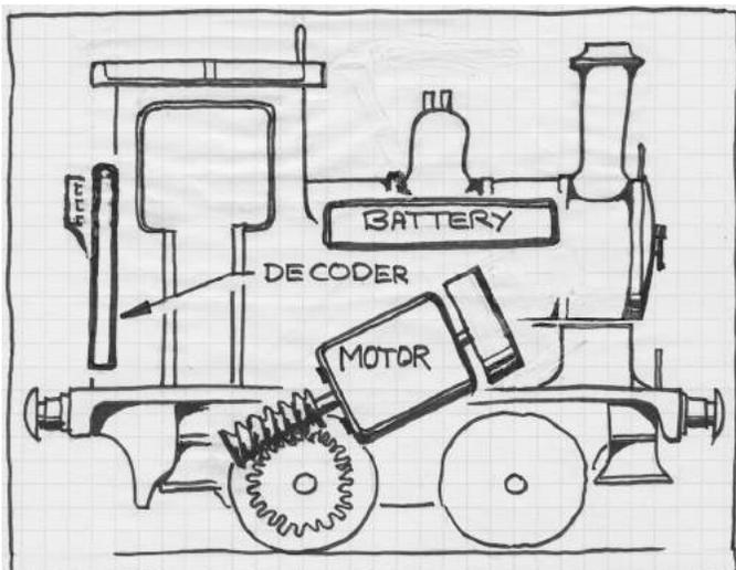
[35] Phantom side view of Loco showing Motor, Battery and Decoder.
