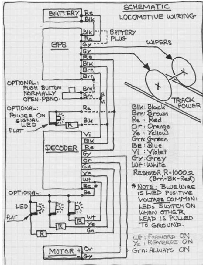
[15] Complete tank loco S-CAB wiring diagram.
