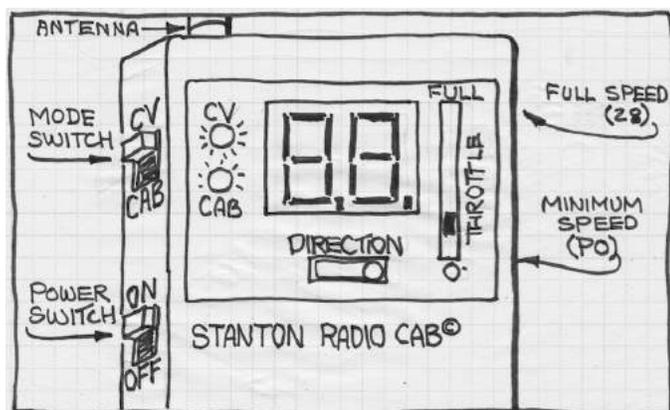
[9] Upper face of S-CAB Throttle showing Tier 1 controls.
