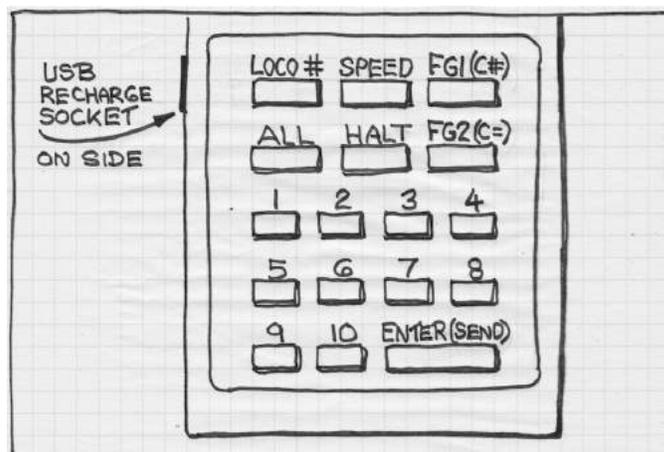
[10] Lower face of S-CAB Throttle showing Tier 2 and Tier 3 controls.
