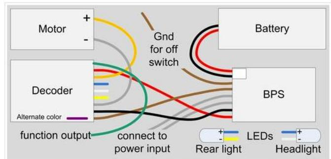
Wiring diagram for a non-sound decoder. Also applies for sound decoder with addition of a speaker.
