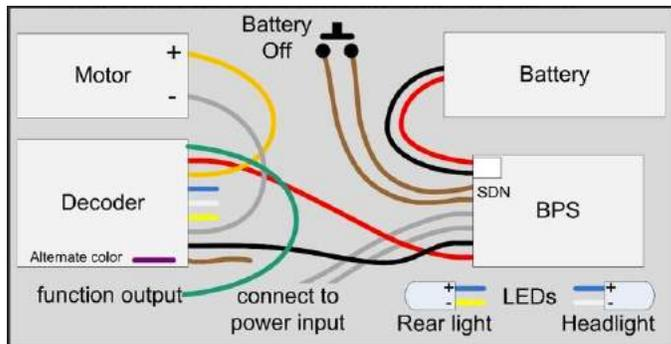
[12] *Wiring for PBNO to manually push Battery OFF*
