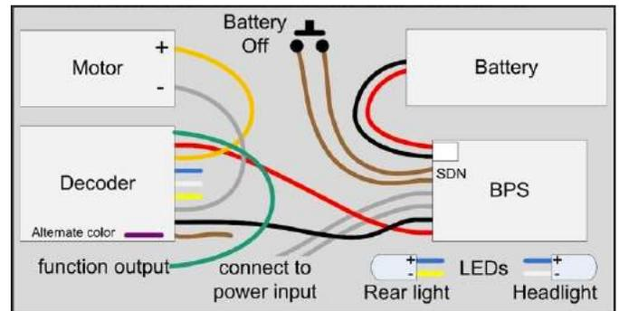
[12] *Wiring for PBNO to manually push Battery OFF*
