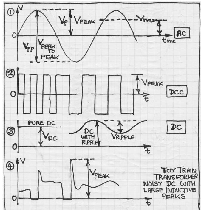
[43] Comparative drawing of the various power supply waveforms. Note the wild behaviour of a toy train set transformer.
