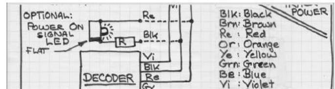
[45] Section of wiring diagram showing power-ON LED. It is connected to the wires running from The Battery to the BPS.
