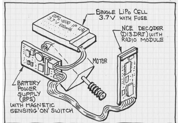
[8] Relative positions of S-Cab components with locomotive removed.
