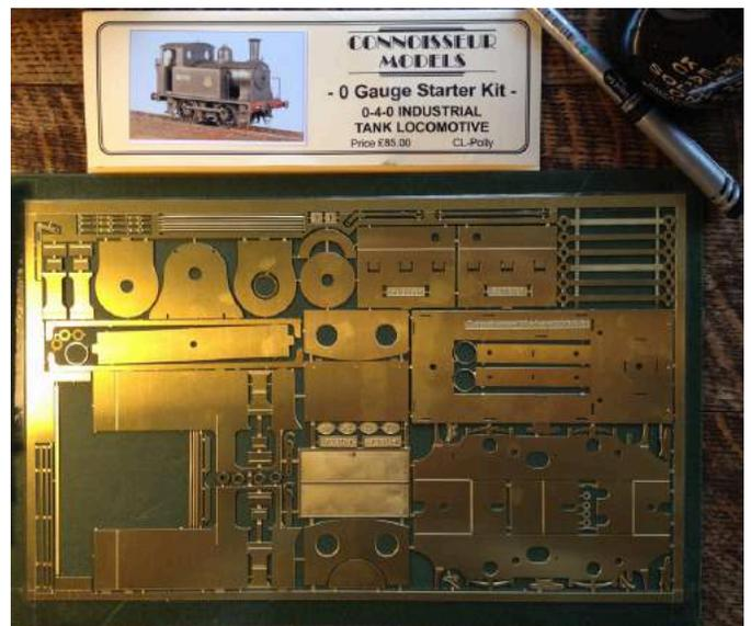
[5] Brass etched fret for O Gauge Starter Kit 0-4-0T. The boiler has been removed by Jim McGeown and pre-rolled.
