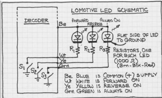
[48] Each decoder LED is tied to a transistor which acts as a switch to turn ON/OFF the corresponding LED.
