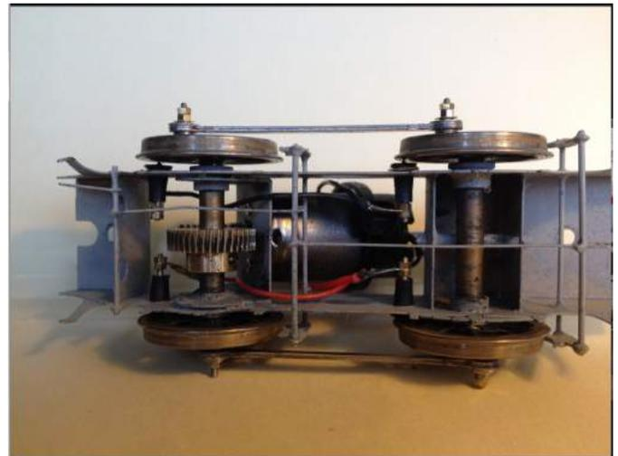
[36] Underneath of loco showing Slater's Plunger Pickups at wheel rims.
