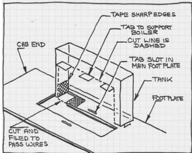
[21] Side tank showing metal to be cut out along the dashed line.
