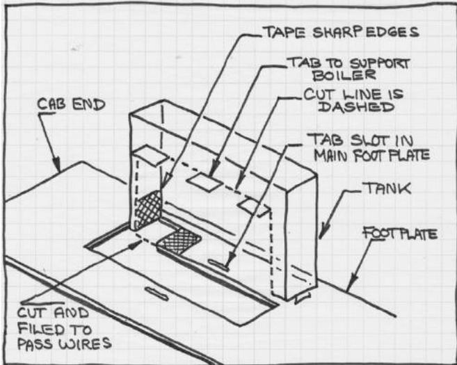
[21] Side tank showing metal to be cut out along the dashed line.
