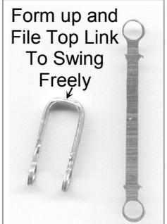
As the buffer head is projected on a longer than normal shaft and the coaches have a long wheelbase you may have coupling up and buffer locking problems on curves and point work. So I have included two different lengths of coupling centre and I suggest you experiment and mix and match to suit your layout. Also included on the etch is a pair of plain hooks that can be used with three link couplings if you wish.
