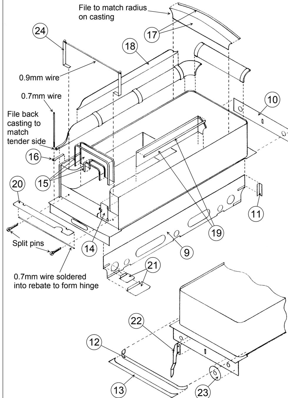
Now using a curved scalpel blade and fibreglass brush work around the solder joints scraping back and burnishing to reveal a sharp line at the joints with no gaps. On the prototype the flares were stepped out from the tender sides with a distinctive joint line. Trim the ends of the side flares to match the sides. The masters for the flares were made over length to accommodate shrinkage in the mould.
