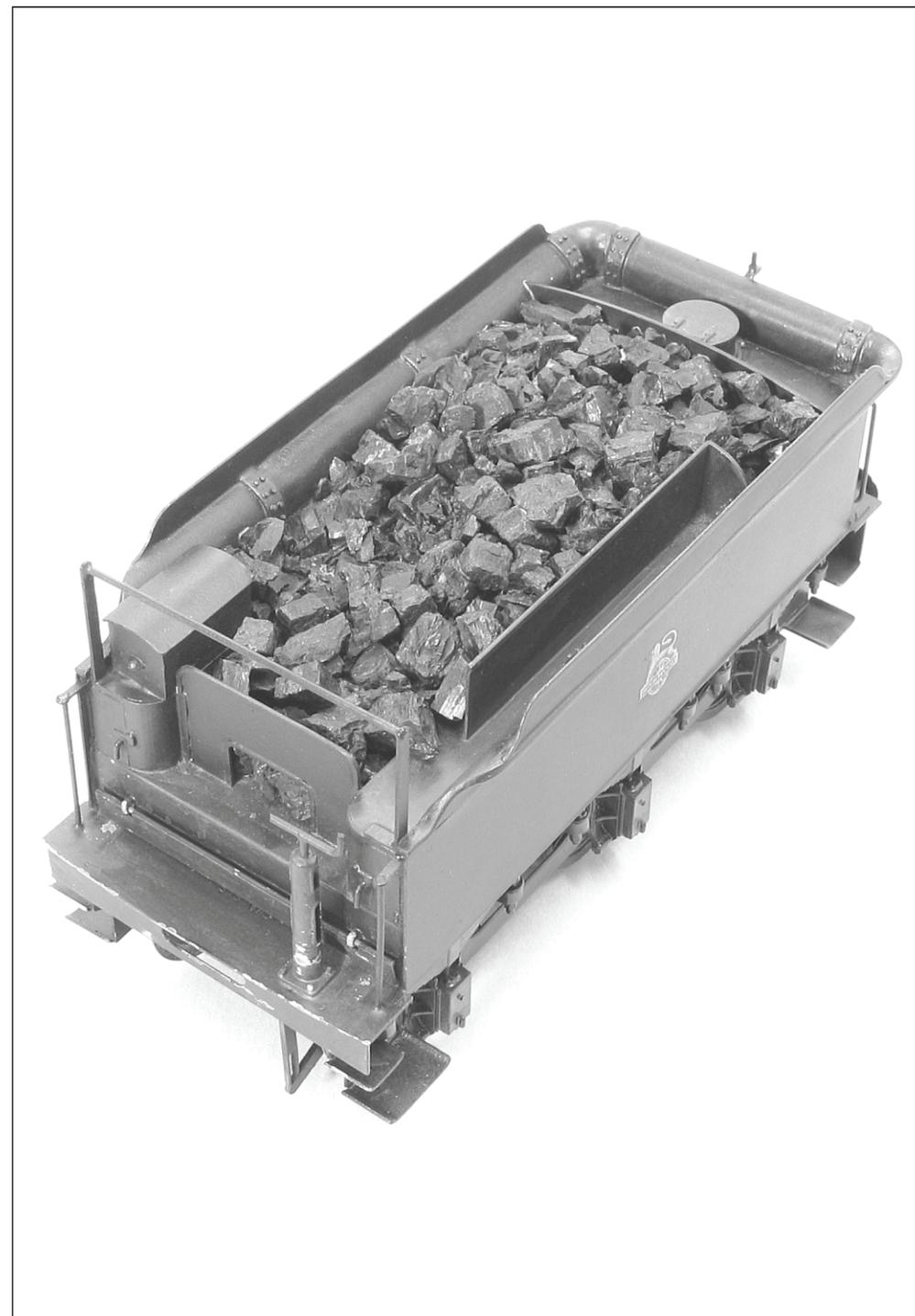
The chassis is fixed to the body using two 6BA screws into the captive nuts that you soldered to the footplate as one of the first operations. No matter how careful you are in building the tender body you will probably have built in a slight twist. It is important that the body does not twist the level chassis out of square so I recommend only locking tight one screw leaving the other slightly backed off.
