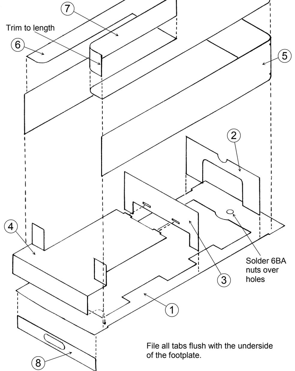
File all tabs flush with the underside of the footplate.
