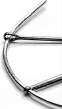
Fit the handrails made from 0.7mm brass wire. In common with the other kits in my range I have included split pins to support the handrails. These are fairly easy to use and their appearance can give a better representation of the prototype handrail supports than some of the turned brass alternatives.
