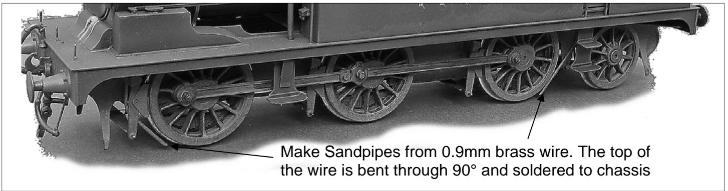
Make Sandpipes from 0.9mm brass wire. The top of the wire is bent through 90° and soldered to chassis
