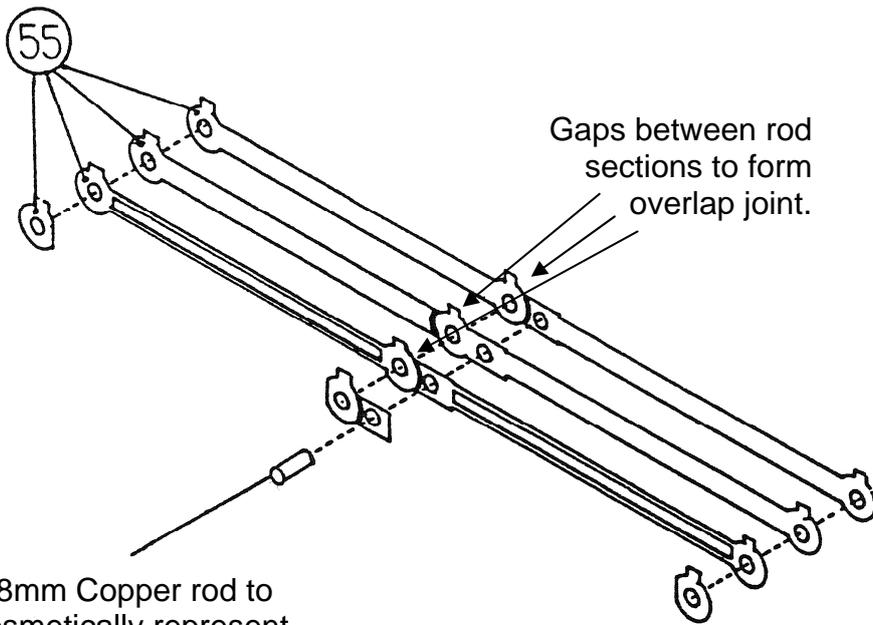
1.8mm Copper rod to cosmetically represent knuckle joint pin
