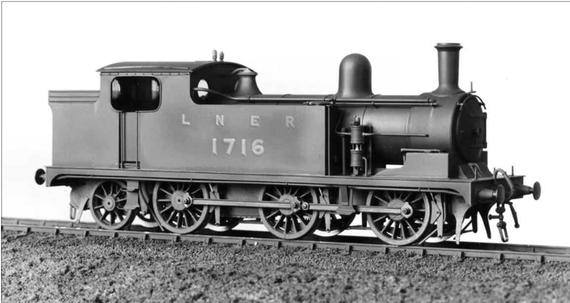
**Prototype.** This class of 20 locomotives were built from 1902. Although mainly intended for mineral and freight train working all of the class were built with Westinghouse brakes. They proved useful on passenger trains and lasted until 1962.
