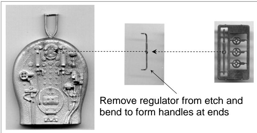
Remove regulator from etch and bend to form handles at ends
