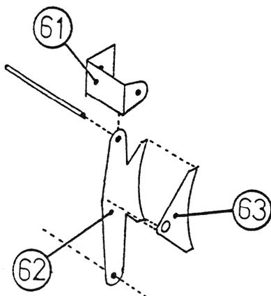
**Part 61, Hanger Brackets, Parts 62 & 63, Brake Blocks and Hangers.** Fit lengths of 0.9mm brass wire across frames then thread brackets & hangers onto this. Solder bracket to side frame and hanger to wire so that the blocks line up with the wheel fronts. Fit wire through lower hanger holes.
