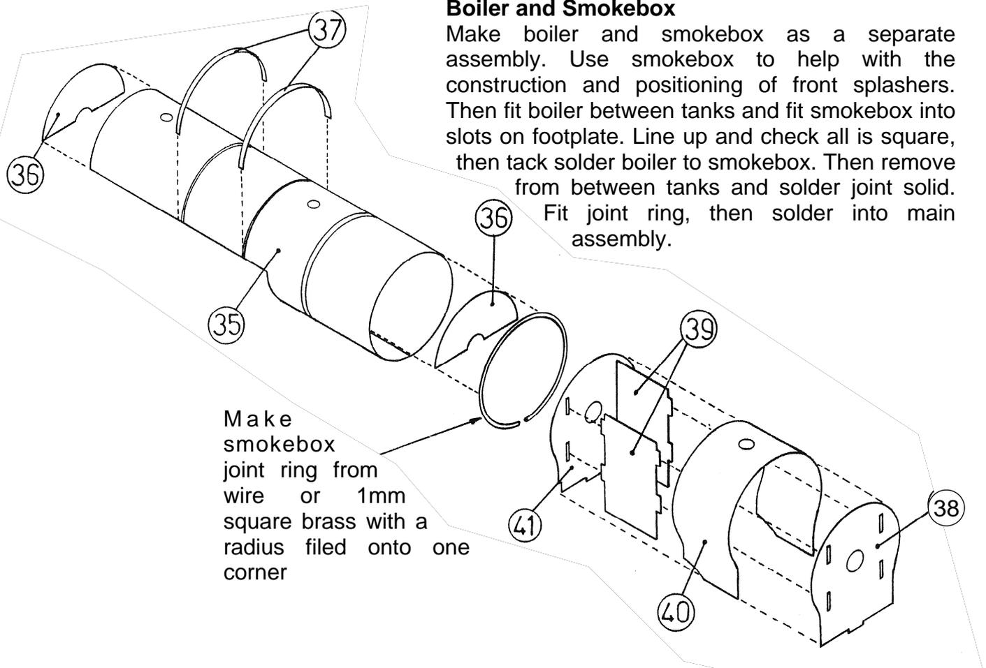
Fit joint ring, then solder into main assembly.
