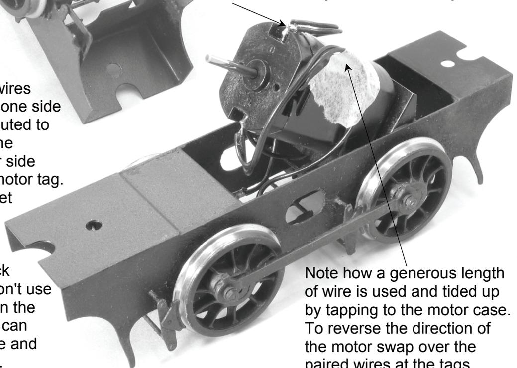
Note how a generous length of wire is used and tidied up by tapping to the motor case. To reverse the direction of the motor swap over the paired wires at the tags.
