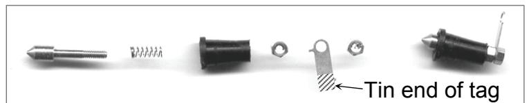
way I can solder the tinned end of the electrical wire very quickly onto the tag with no risk of heat getting to the plunger. I prefer to fit a separate length of electrical wire to each pickup and join the wires as I terminate them at the motor tags. I find that this is neater and easier than trying to link the pickups on each side together using jumper wires.
