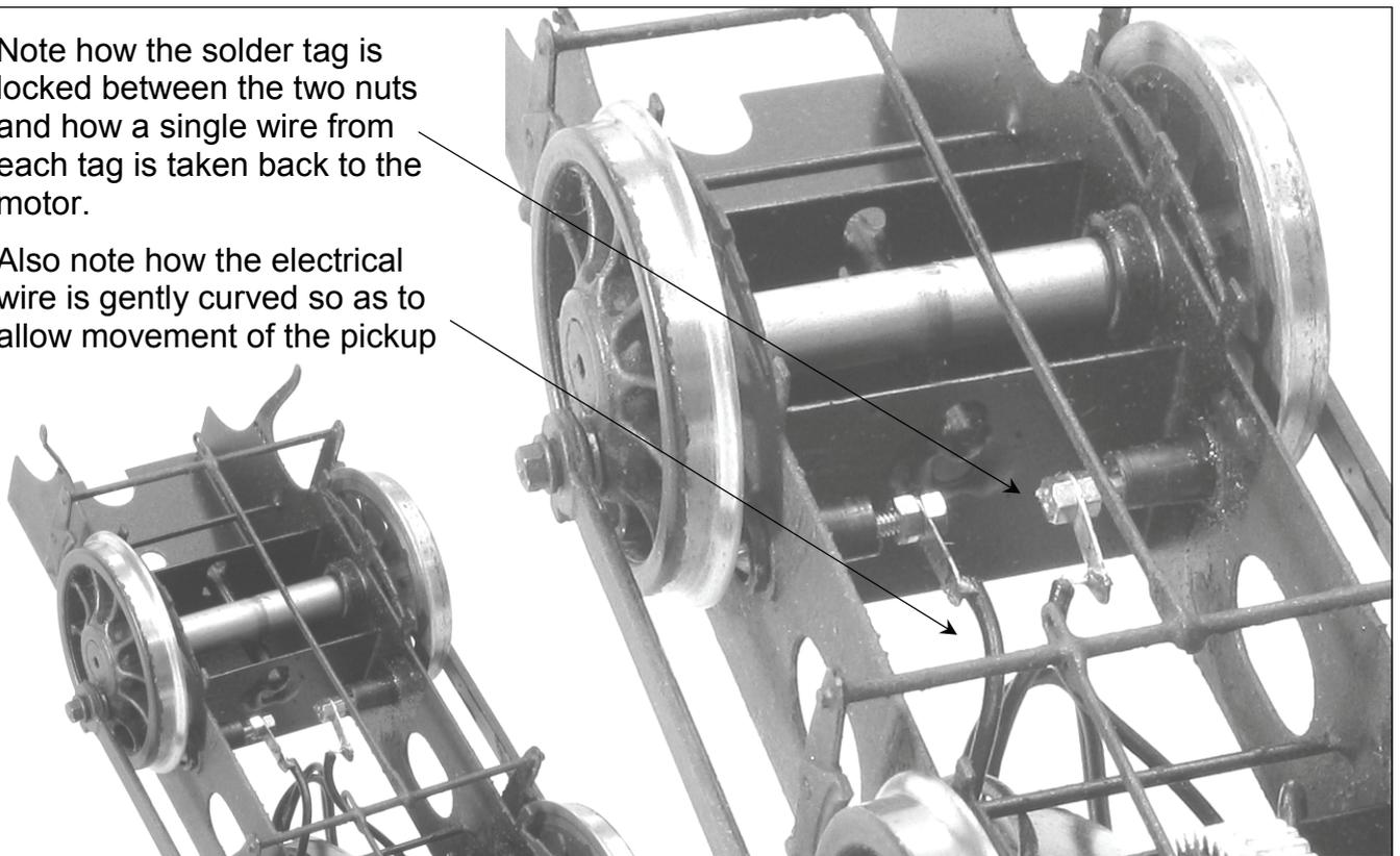
Note how a single wire is taken back from each pick up and then paired together at the motor solder tag. For a six wheeled loco you would have three wires on each tag but make sure you strip the wire insulation evenly and solder neatly.
