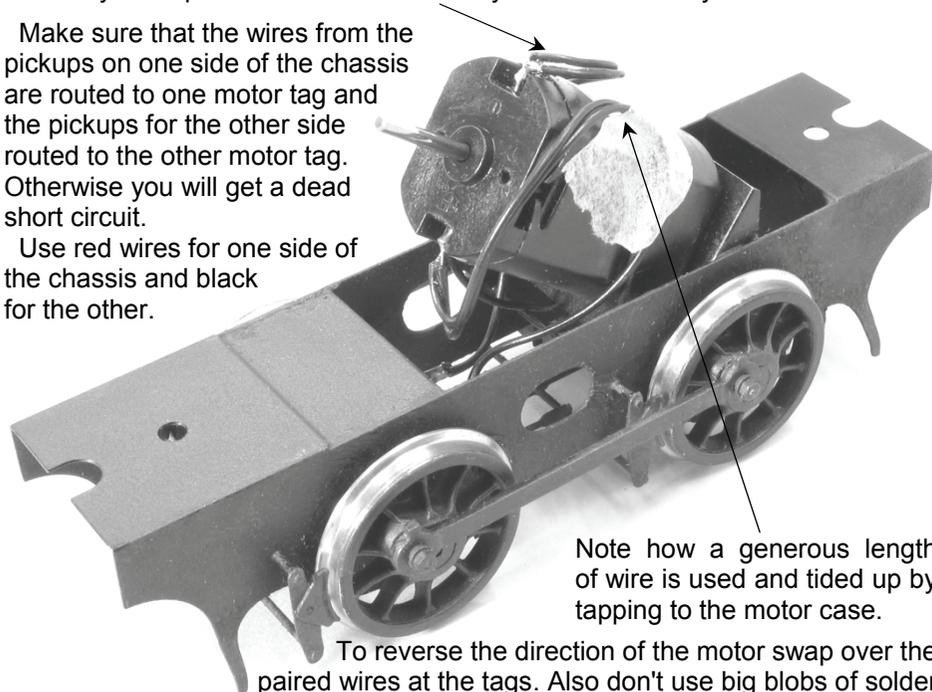
Note how a generous length of wire is used and tidied up by tapping to the motor case.
