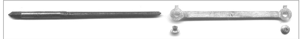
We now have to reduce the length of the bush to prevent sloppy side play in the rods. Place a bush onto a block of wood then place a coupling rod face down over the bush. By pressing down on the rod with your finger you should be able to gently file the bush until it is 0.010" to 0.015" proud of the rod. These bearing bushes are not soldered into the rods but locked onto the crankpin with a nut and washer. So it is important that they will revolve freely in the holes in the rods.
