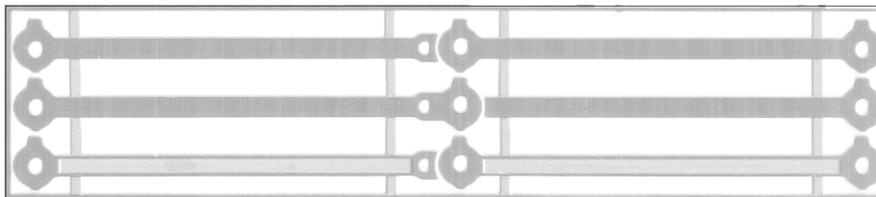
I decided to make the best of my successes and joined the two brass parts together with five good spot joints. I was very pleased with myself and at the strength of the joint. That was until I realised that the two parts were joined together out of square. Although the parts were propped in position with blocks of wood I had managed to move them out of position when I was feeding the solder into the joint with my left hand.
