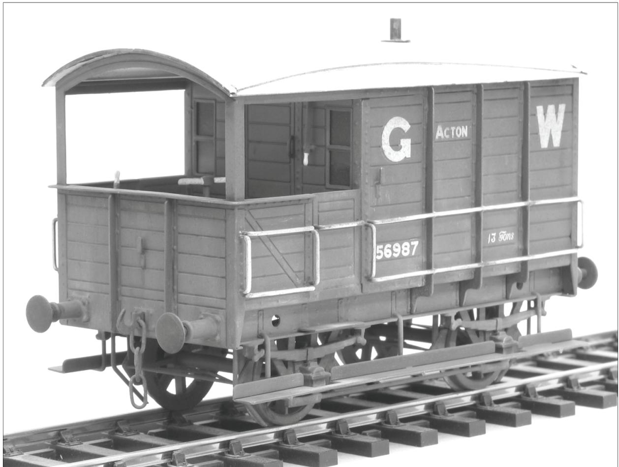
**Prototype.** Twelve of these short wheelbase vans were built in 1898 originally for working in the London area and stationed at Acton. They were 9 foot wheelbase and 16 foot over headstocks. It can only be assumed that space for headshunts and sidings was at such a premium in the Metropolis that such a short brake van was required to fit into them. A situation that is familiar to many of us on our own layouts. These vans lasted into British Railways days.
