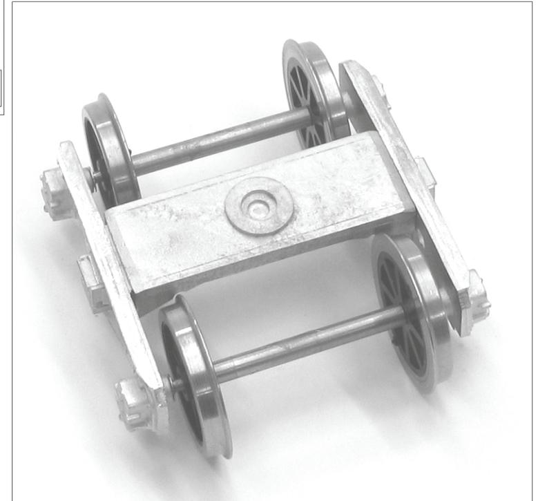
9. Assemble the bogies. Drill out the holes in the side frames 2.6mm to accept the brass bearing cups. You may find that the holes are slightly out of square so put a little sideways pressure on the drill to square them up. Keep checking the depth of the hole with a bearing as you don't want to drill too deep and come through the front of the axle box.
