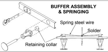
any white metal casting more accurate). Then fit the shanks through the buffer body, snip off some of the narrow end of the shank to leave just over 1mm from the step, and solder a retaining collar onto the shank.
