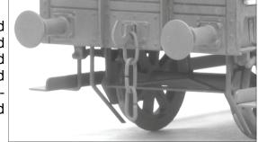
hole in the coupling hook. I reinforce the joint of each link with a spot of 60/40 solder.
