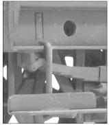
Fit end window rainstrips (parts 10) wide ones to the top and narrow to bottom. Form up the lamp irons (parts 11) and reinforce the folds with 60/40 solder. Fit the lamp irons to the body sides and ends noting that there are etched marks to help with positioning.
