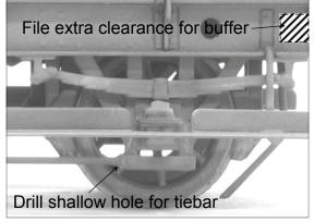
Slip wheel sets with the axle guards on between the solebars and tack solder each axle guard with low melt solder to the solebar (the cut-outs in the footboards will help with positioning). Check that the axles are parallel and the wheel centres are about 91mm apart. Place the van onto a flat surface and adjust if necessary by re-soldering each axle guard until the van sits without rocking, when happy solder solid. If necessary drill through the two horse hooking holes in the solebars to clear.
