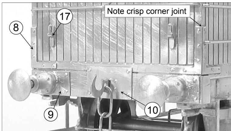
Fit the handrails, made from 0.7mm brass wire. I find some strips of thin card (0.8mm-1mm thick) useful to help space out the handrails from the body as they are being soldered into place. I fitted the vertical doorway handrails first (make sure that the ends of the wire doesn't come too far inside or this will prevent you fitting the veranda floor later) and then the horizontal ones.
