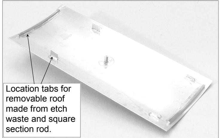
10. Now for the roof. I have pre-rolled this in my rolling bars but you may have to work it a little with finger and thumb to get it to the exact profile. Mark out the roofs centrelines and drill a hole for the chimney.
