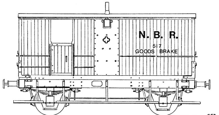
NBR lettering position and livery, Bodywork etc - dark grey. Other components as LNER
