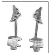
6. Solder brake blocks (parts 14) to brake hangers (parts 15) making up four left hand and four right hand. Using a round file put cut outs into the bases of two pairs of hangers that will form the outer brakes. This is to provide clearance for the buffer springing wire.
