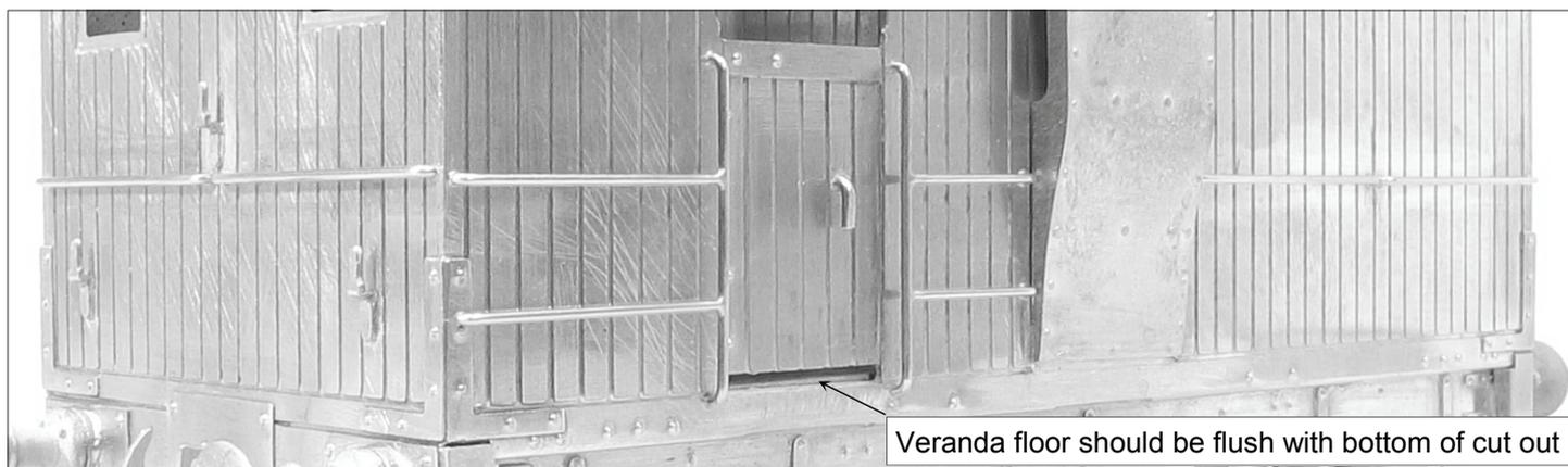
4. Fold through 90° the bottom edge of the solebars (parts 11). The tabs towards the ends of each solebar set the height of the veranda floor. Its a good idea to temporarily fit the solebars into their slots and offer the floor into place. The top surface of the floor should be flush with the bottom of the below door cut out. If required file the tops of the tabs to achieve this.
