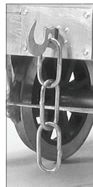
Pass the coupling hook through the buffer beam slot and retain it with a length of spring wire. Polish the centre of this wire with emery cloth first so that you can solder it to the coupling hook shank once you are happy that the buffers spring freely. Because of tight clearances they will only depress about half way in.
