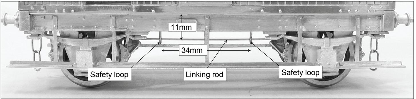
Using 0.7mm brass wire form up a rod to link the inner brake yokes and solder into position so that it runs parallel to and 11mm below the wagon floor. Again using 0.7mm brass wire form up two safety loops for this rod and solder to the underside of the floor 34mm apart. The centre footboard support will give a good visual guide for the vans centre line.
