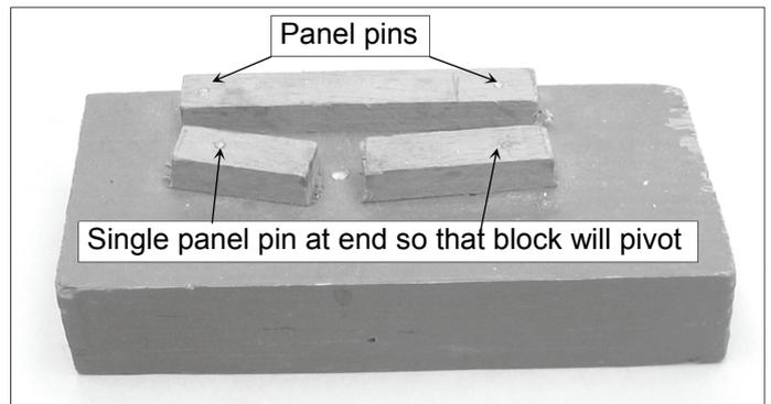
I suggest that you hand drill the hole with the drill bit held in a pin vice so that you have control over the depth of the hole. If you want to speed the job up by using an electric mini drill I would suggest drilling only  $\frac{2}{3}$  of the depth with this and then finishing off by hand so that you can check the depth with the bearing. You don't want to have to patch the axle box with low melt solder because you have come through the front.
