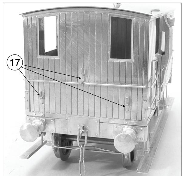
Generously tin with 145° the top and bottom of the etched rebate panel and adjacent brass timbers. Fit the cast ductet into the etched panel and run a good fillet of low melt solder along the top and bottom edge. Then using a knife blade and fibre brush scrape back and blend the casting into the etched top and bottom timber.
