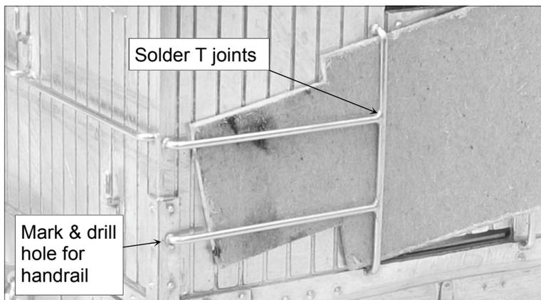
The horizontal doorway handrails join the vertical ones as a T joint. I spot-soldered these joints using 60/40 electrical solder as this gives a stronger joint than using 145° solder. Use plenty of flux and make sure the solder runs all around the joint. You will have to mark and drill a hole in the corner strapping for the bottom horizontal handrail. Also note that some vans had extra horizontal handrails fitted by the LNER (see scale drawing) and if fitting these mark and drill extra holes.
